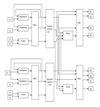
Fig. 8: Trellis check node unit decoding architecture with permutation network
