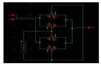
Fig. 6: Multiplexer for the permutation network
