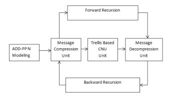
Fig. 1: Block diagram of trellis based decoding architecture
