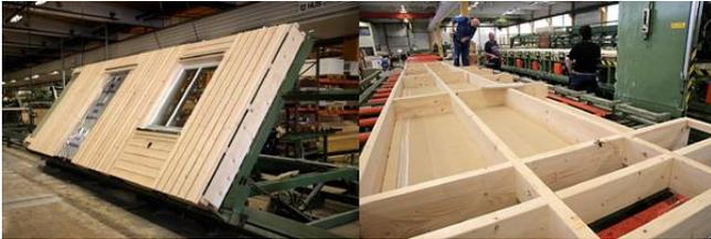
Fig. 1: Manufacture of panel construction system [33].
