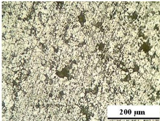
**Fig. 9b:** Microphotograph illustrates the microstructure of NZ for see water SFSW (1460 rpm, and 60 m/min)
