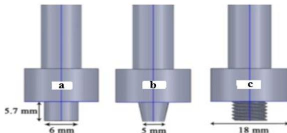
**Fig. 1.** Tool pin shape (a) round pin (R); (b) conical pin (C); and (c) thread pin (T).
