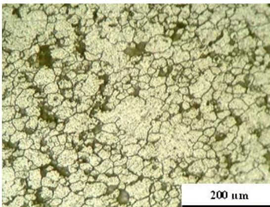
**Fig. 9c:** Microphotograph illustrates the microstructure of NZ for oil SFSW (1460 rpm, and 60 m/min)
