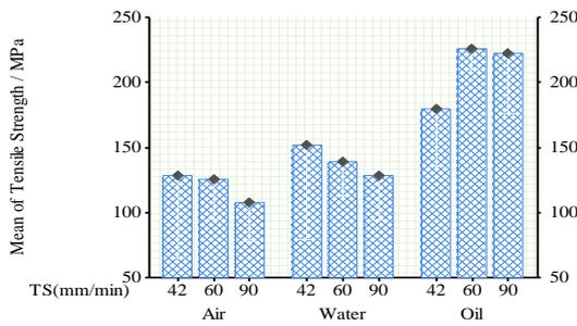
Fig. 4: Plots illustrate the interactions between cooling media and travel speed versus tensile strength.
