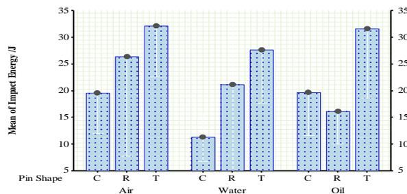
Fig.6a: Plots illustrate the interactions between cooling media and pin shape versus impact energy.
