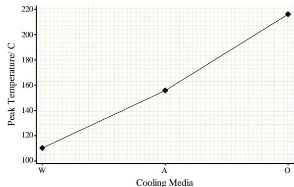
Fig.8. The effect of the cooling media on the peak temperature of the welded parts.
