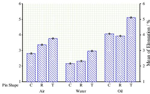
Fig.5a: Plots illustrate the interactions between cooling media and pin shape versus the welding ductility.
