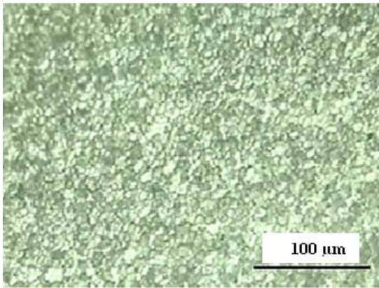
**Fig. 9a:** Microphotograph illustrates the microstructure of NZ for CFSW (1460 rpm, and 60 m/min)
