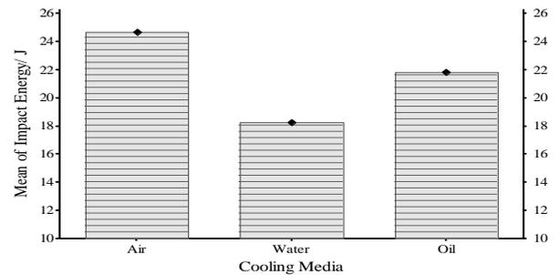
Fig.7. The effect of cooling media on the impact energy.
