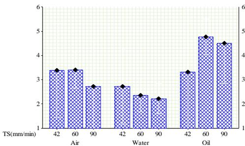
Fig.5b: Plots illustrate the interactions between cooling media and travel speed versus the welding ductility.
