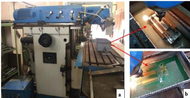
**Fig. 2.** SFSW set up, (a) the milling machine, and (b) close up shows the submerged FSW.
