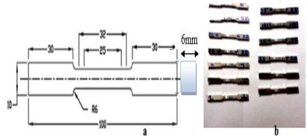
**Fig. 3.** (a) ASTM Sub-Size specimen for tensile test [13]; and (b) photograph illustrates the prepared tensile specimens.
