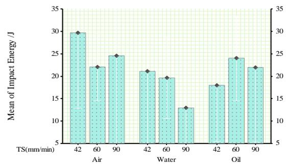
Fig.6b: Plots illustrate the interactions between cooling media and travel speed versus impact energy.
