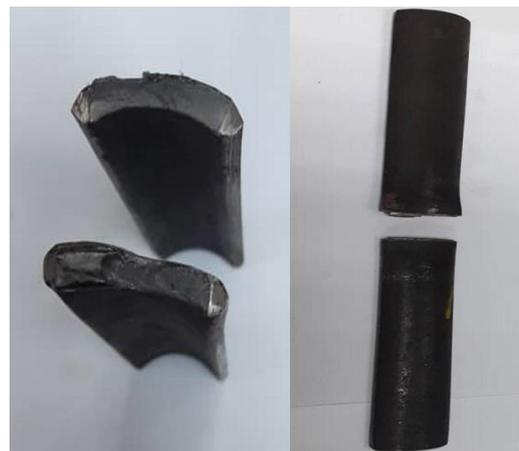
**Fig. 7:** Nick break test of the welded specimen
