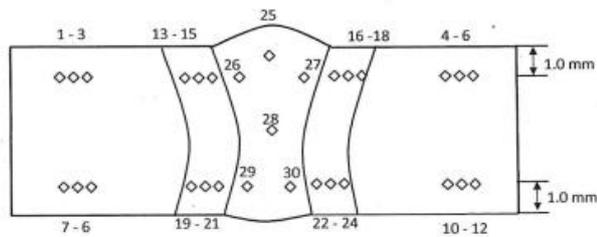
Fig. 8: Vickers hardness test of the welded specimen
