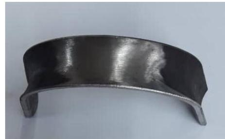
**Fig. 6:** Side bend test of the welded specimen
