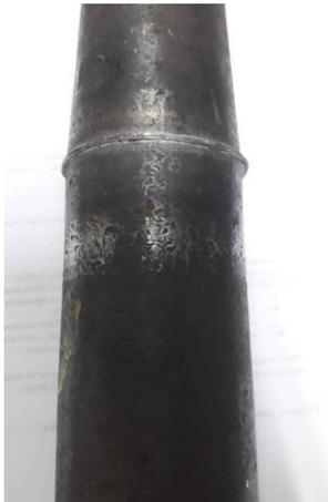
**Fig. 4:** Uniform bead and full penetration
