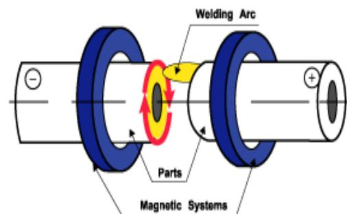
Fig. 1: Two pipes are set coaxially in MIAB welding
