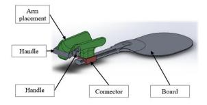
Figure 4: Model of the new radial arm board.
