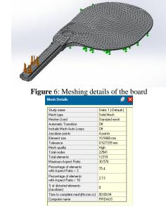
Figure 7: Meshing details of the board.
