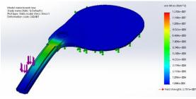
Figure 9: von Mises stress of the board.
