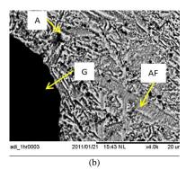
**Figure** 4: (a) Microstructure and (b) SEM observation of Nb-ADI sample showing G-graphite, A- retained austenite AF- acicular ferrite platelets.
