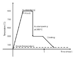
Figure 1: The schematic diagram of the austempering heat treatment.
