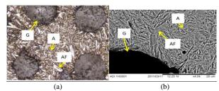
**Figure** 3 : (a) Microstructure and (b) SEM observation of ADI sample showing G-graphite, A- retained austenite, AF - acicular ferrite
