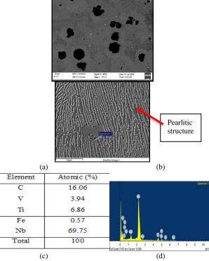
**Figure** 2: SEM result of 0.5 wt % Nb-DI at (a) lower magnification (b) higher magnification, and (c) composition and (d) peak of element of at sparked spectrum.
