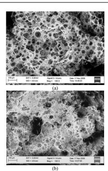
**Figure** 5. SEM Fractograph of the sample after tensile test for (a) ADI and (b) Nb-ADI
