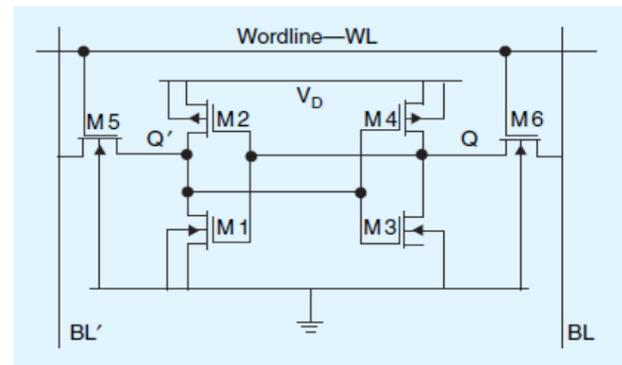
Fig. 3: Schematic of Standard 6T FinFET SRAM Cell.
