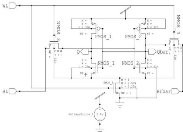
Fig. 5: Design of Finfet Based SRAM Cell with Fine Grain Power Gating.
