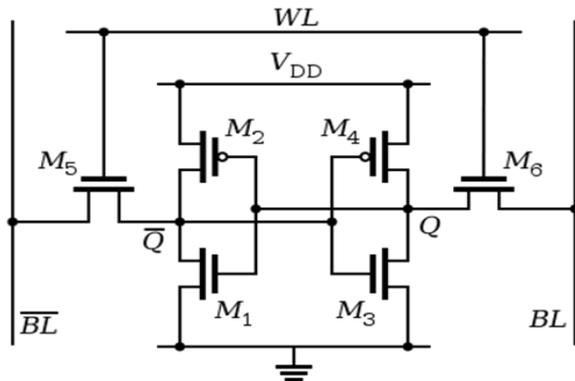
Fig. 1: An Example of A Typical 6T SRAM Cell [18].
