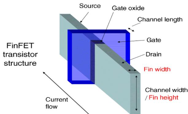
Fig. 2: The basic schematic structure of FinFET Transistor [18].
