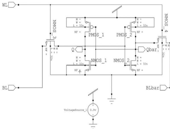
Fig. 4: The layout of FinFET based standard 6T SRAM cell in S-edit.
