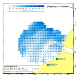
Figure 6: Surface current field from the Taiwan coast near Taipei in 2015, with the average time for acquiring the data was set to 30 min.
