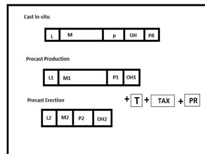
Fig. 4: Schematic comparison of relative economies between cast in-situ and precast concrete construction
