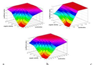
**Fig. 4.** Sugeno-model nonlinear transformation. a) *a*<sub>1</sub>=0, *a*<sub>2</sub>=0, *a*<sub>3</sub>=0.5; δ) *a*<sub>1</sub>=3,5; *a*<sub>2</sub>=8; *a*<sub>3</sub>=0,5; B) *a*<sub>1</sub>=3,5; *a*<sub>2</sub>=8; *a*<sub>3</sub>=0,5
