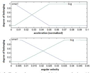
Fig. 3. The form of representation of the input term for the variables  $\alpha$  and  $\beta$
