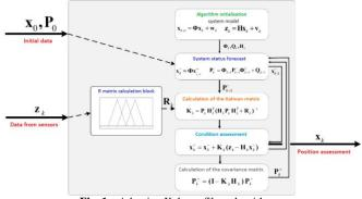
Fig. 1. Adaptive Kalman filter algorithm
