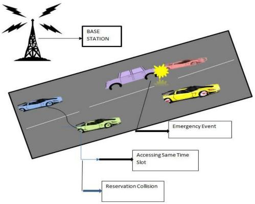
Fig. 1: Vehicular Ad Hoc Network Architecture.
