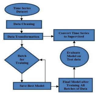
Fig. 3: LSTM Recurrent Neural Network Modeling Process.
