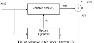
Fig. 4: Adaptive Filter Block Diagram [39].
