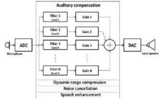
Fig. 3: Filter Bank Block Diagram for Hearing Amplification [40]. the Filter Bank For Hearing Amplification Is Designed Such That the Raw Analog Signal Is First Converted Into A Digital Format. Subsequently, Processes Inclusive of Auditory Compensation, Dynamic Range Compression, Noise Cancellation, and Speech Enhancement are Achieved, Through Separating the Frequency Components Via Filters Prior to Combining Them. after This, the Processed Signal Undergoes Digital to Analog Conversion.
