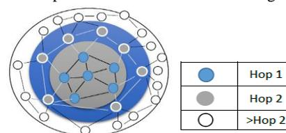
Fig. 3: Fish Eye State Routing Protocol
