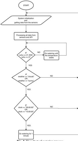
Fig. 4: Flowchart of watering process
