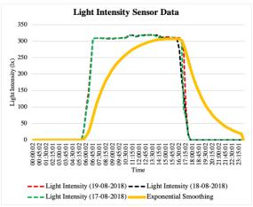
Fig. 11: Graphic of light intensity sensor data reading
