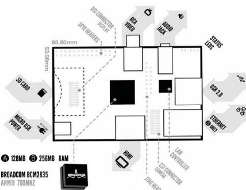
Fig.3: Raspberry Pi Connection
