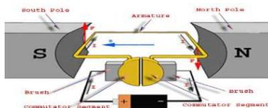
Fig.4: DC Motor Architecture
