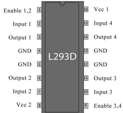
Fig.4: Pin Diagram of L293d motor driver
