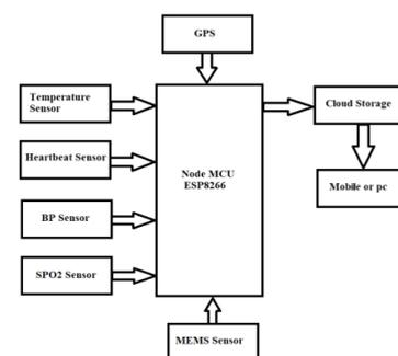
Fig 1: Block diagram autonomous health monitoring
