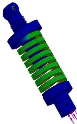
**Fig. 8:** stress output of solid square cross section helical spring.
