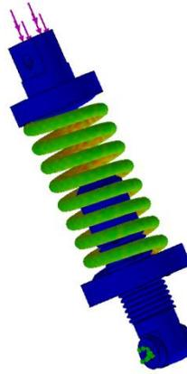
**Fig. 9:** stress output of hollow circular cross section helical spring
