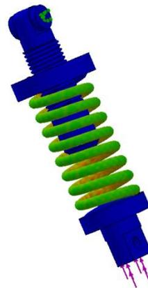
**Fig. 7:** stress output of solid circular cross section helical spring
