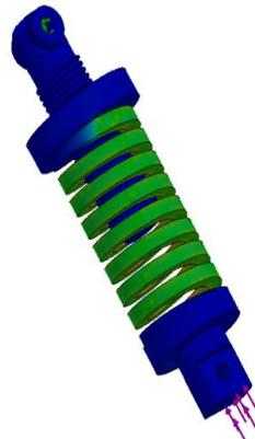
**Fig. 10:** Stress output of hollow square cross section helical spring
