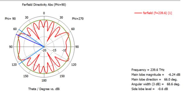
**Fig. 9:** Polar Plot of the Frequency 240 THz.
