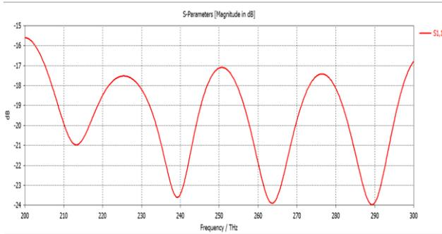
**Fig. 5:** Amplitude of the Reflection Coefficient (I.E., Scattering Parameter  $S_{11}$ ) at the Input Port of the Horn Nanoantenna.
