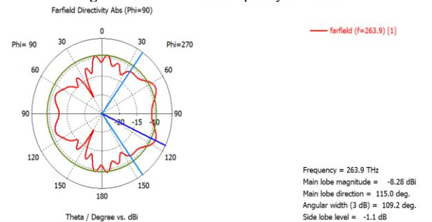
**Fig. 10:** Polar Plot of the Frequency 264 THz.
