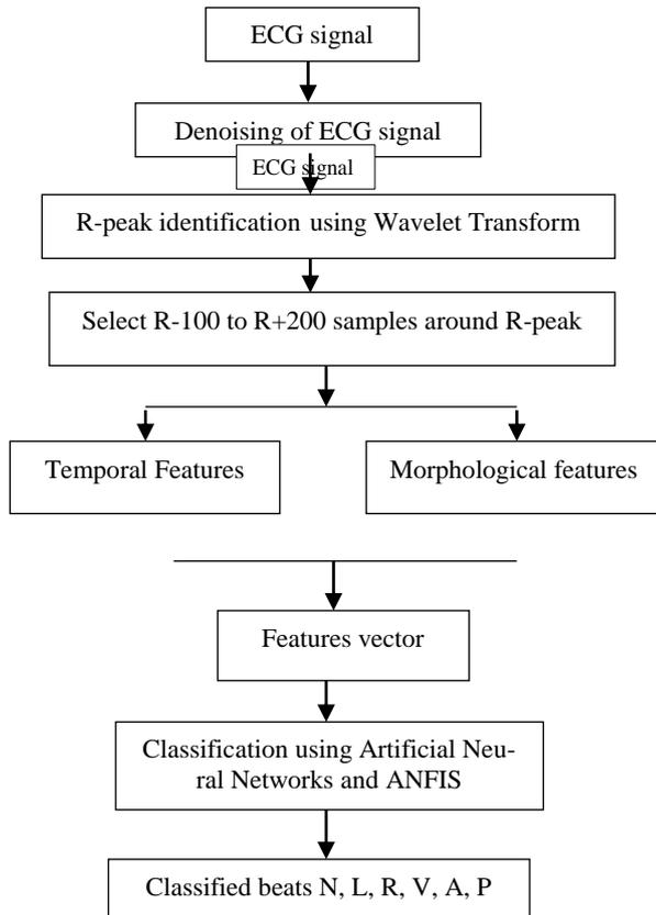
Fig. 1: Block diagram for classification of cardiac Arrhythmias
