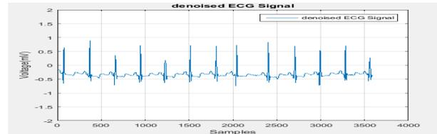
Fig. 3: Preprocessed ECG signal (Record 100 of ten seconds duration)
