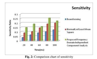
This chart explains about the sensitivity ratio of two existing methods and one proposed method. The sensitivity ratio of its range is been explained using number of packets in X axis and the sensitivity ratio of the process in Y-axis. While analyzing and comparing proposed method with existing method, proposed Method shows maximum value of sensitivity ratio from 0.149 to 0.223. Whereas, the other two existing methods involves more sensitivity ratio.
