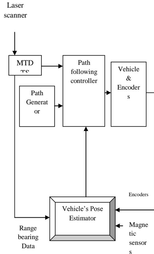
Fig. 4: System model for Mobile Robot
