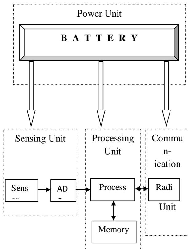
Fig 2: Sensor node architecture.
