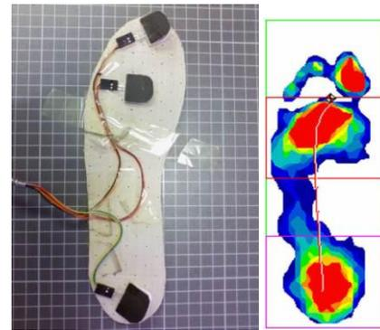
(a) sensor placement on the in soles., (b) Pressure distribution on foot [6]
