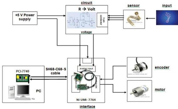
Fig. 3: Schematic diagram AAFO interfacing system [17]
