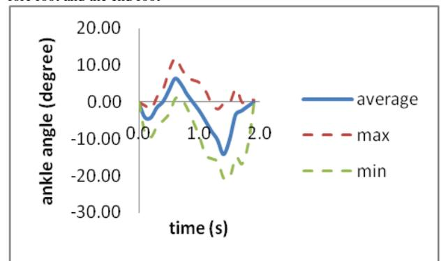
(b) The range of ankle angle of rotation results based on rotary encoder at the ankle joint
