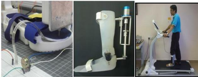
(a) System overview of AAFO includes sensors and DC motor, rotary encoder and lead screw mechanism placement
