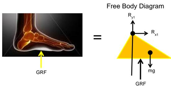
Fig. 1: Free Body diagram of force at ankle joint
