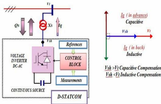
**Figure:** Basic model of DSTATCOM connected to the network
