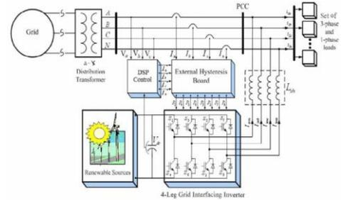
**Figure:** Schematic diagram of the distribution system with renewable energy sources
