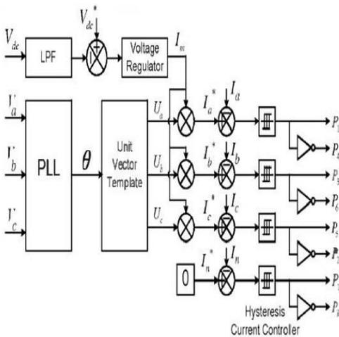
Figure: Block diagram of grid connected inverter Control.
