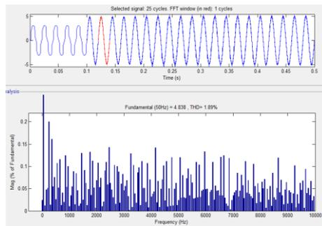
Figure: THD of the source after compensation.
