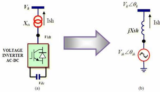
**Figure:** (a) Circuit diagram of DSTATCOM (b) Equivalent circuit of DSTATCOM
