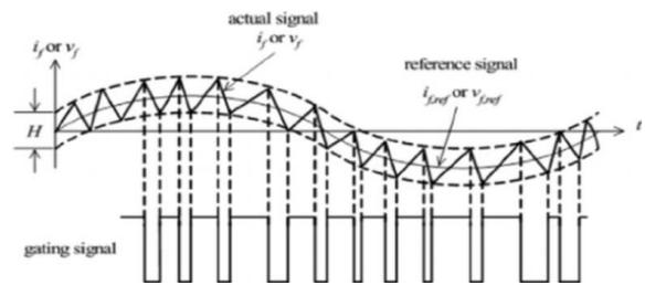
Figure: Waveform of hysteresis current control
