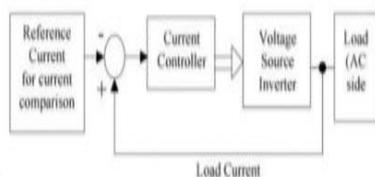
Figure: Block Diagram of Hysteresis current control Technique
