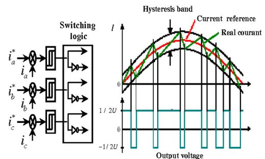
Figure: PWM hysteresis current control and its switching logic
