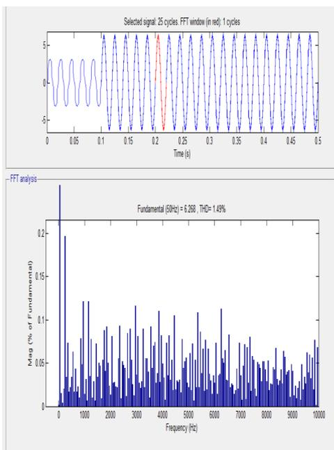
Figure: THD of the source after compensation with fuzzy logic controller.
