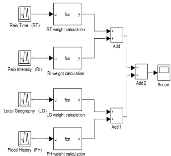
**Fig. 2:** MATLAB Simulink model of proposed FFWS algorithm
