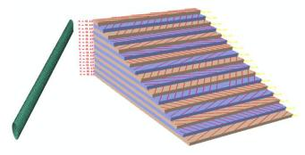
Figure 6: Visualization of ply stack
