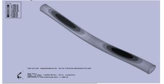
Figure 7: The displacement in y-direction
