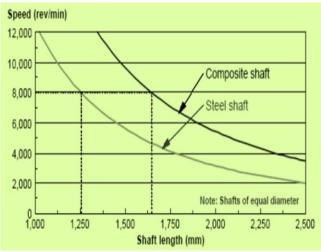
Figure 1: the relationship between shaft's length and the critical speed for both types of drive shafts
