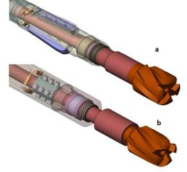
Fig. 1: RSS concepts: a - Push-the-bit; b - Point-the-bit
