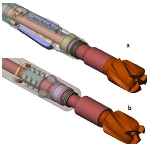
Fig. 1: RSS concepts: a – Push-the-bit; b – Point-the-bit
