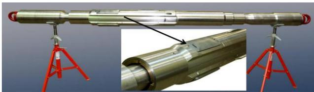
Fig. 2: RUS220 rotary steerable system prototype
