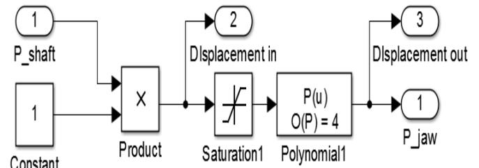
Figure 8: Jaw kinematics subsystem
