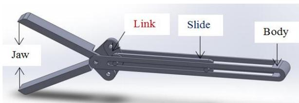
Figure 1: The basic mechanical arrangement of the grasper
