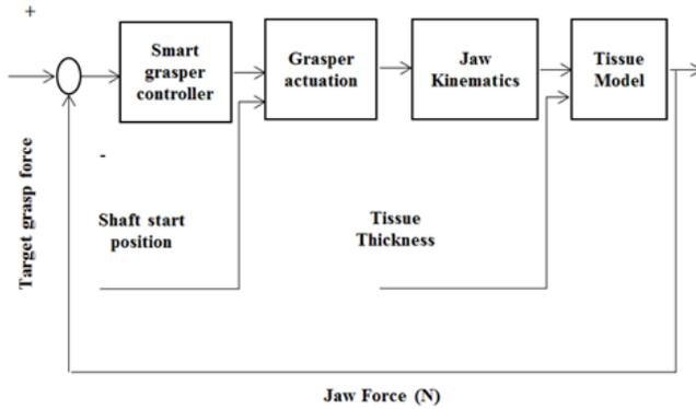
Figure 4: System block diagram of the grasper
