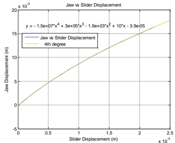
Figure 3: MATLAB Figure of (Jaws Vs Slider displacement)
