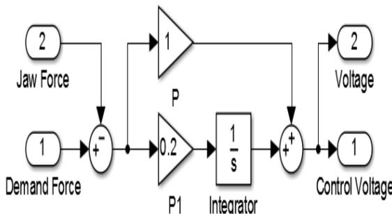
Figure 5: Smart controller subsystem
