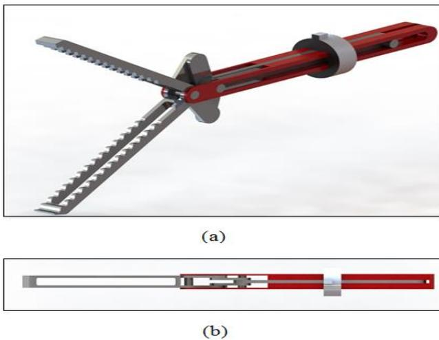
Figure 2: Final model of the laparoscopic grasper in SolidWorks: (a) isometric view of the system (b) Top view of the grasper
