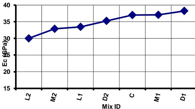
Fig. 9: Static Modulus of Elasticity ( $E_c$ ) Results
