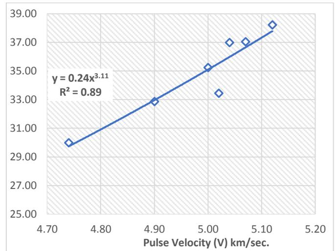
Fig. 13:  $E_c$  vs. V
