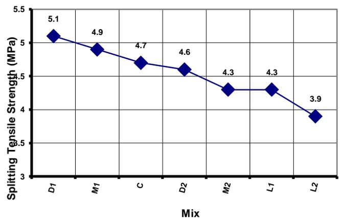
**Fig. 3:** Results of Splitting Tensile Strength
