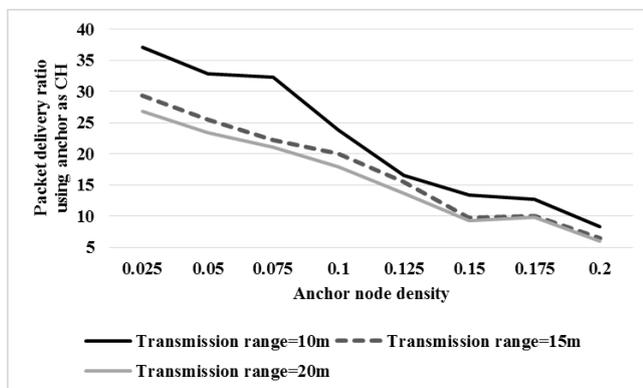
Fig 4 Packet Delivery Ratio (PDR) using Anchors as CH
