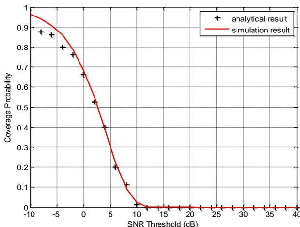
**Fig. 7:** SINR Coverage Probability of Mesh Configuration.
