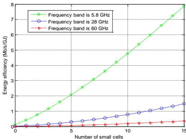
Fig. 3: Energy Efficiency of the Star Configuration for Different Mmwave Bands for 15 Nodes Only.
