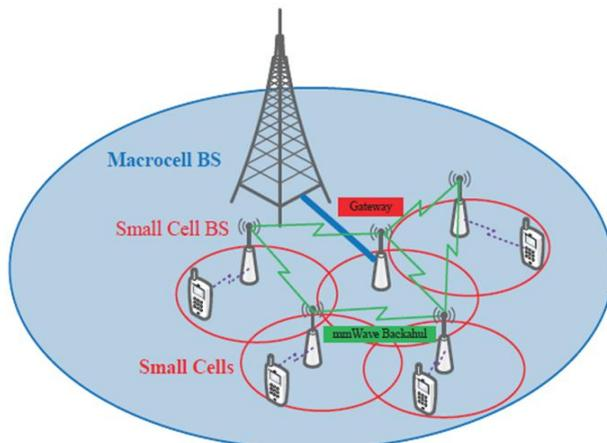
Fig. 1: MM Wave Topology of 5G Network (Niu Et Al. 2017).
