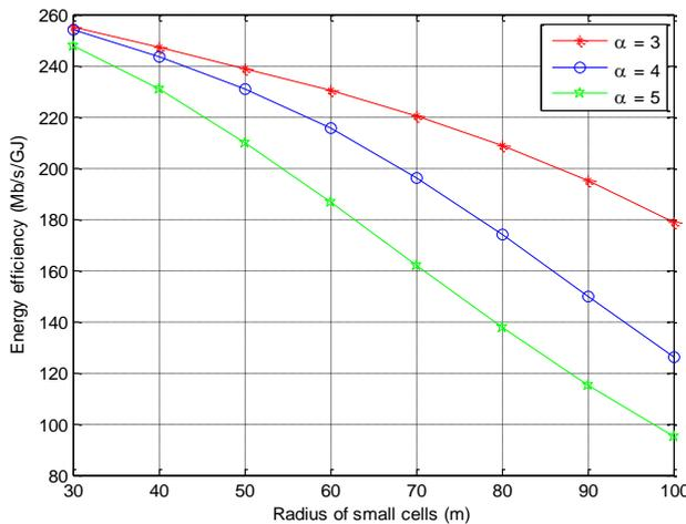
**Fig. 6:** Energy Efficiency of the Mesh Configuration for Different Values of Path Loss Coefficient.
