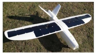
Fig. 14: Completed Aircraft with Integrated Solar Cells.
