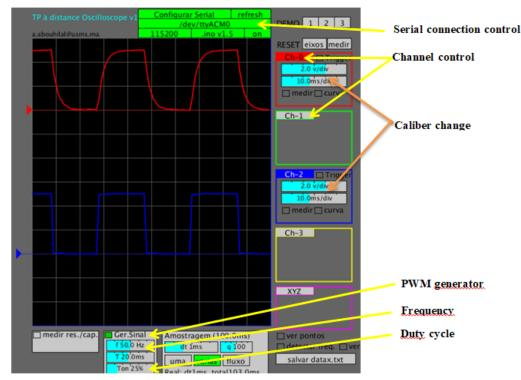
**Fig. 3** : Developed software oscilloscope-GBF
