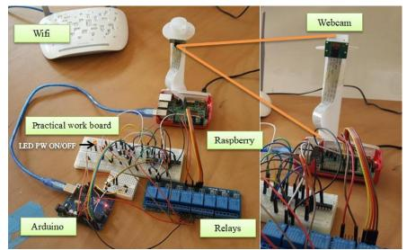
Fig. 4: Realized hardware manipulation
