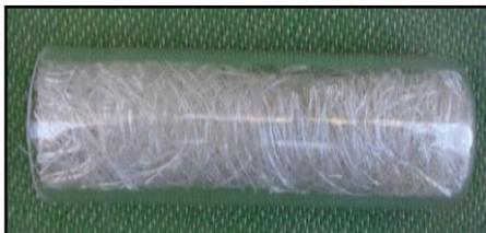
**Fig. 3:** The Fibers in the Glass Mold
