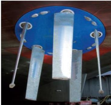
Fig. 1: Voith Schneider Propeller
