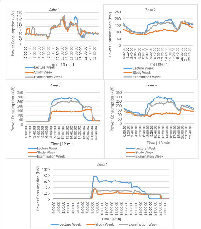
Fig.5: Daily load profile at different zones during distinctive week (lecture, study and examination week)
