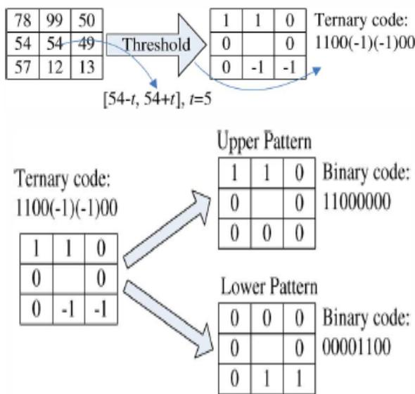
Fig. 2: Procedure of the LTP [6]
