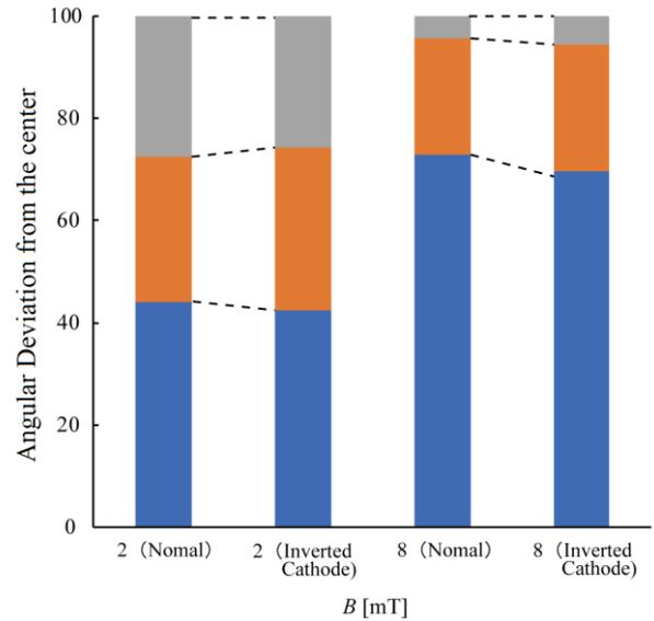
Fig. 6: Comparison of Movement Angles of Cathode Points Due to Change in Magnetic Flux Density
