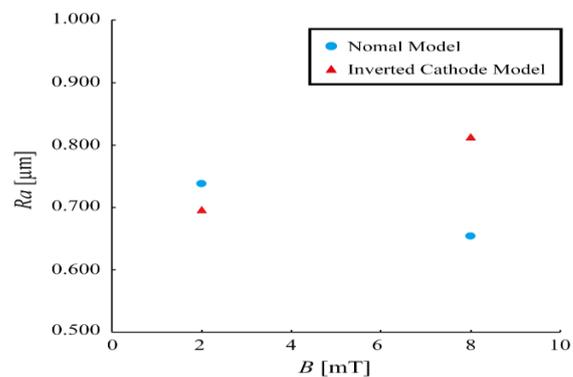
Fig. 8: Comparison Surface Roughness Due to Change in Magnetic Flux Density
