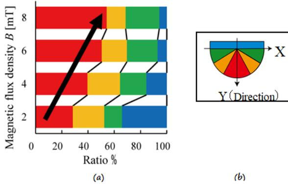
Fig. 1: Effect of Changing Magnetic Flux Density to Direction of Movement of Cathode Spot.
