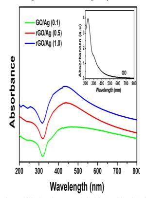
**Fig. 1:** UV-visible absorption spectra obtained for Ag-rGO and Ag-GO nanohybrid solution prepared with different concentration of GO (a: 1.0 mg/ml, b: 0.5mg/ml and c: 0.1/mg/ml). Inset shows a UV- visible absorption spectrum of GO solution.
