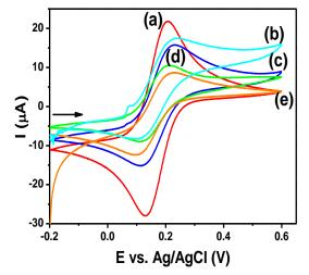
**Fig. 5:** Cyclic voltammograms obtained for bare GCE (a), GO (b), AgNPs-rGO (0.1 mg/ml) (c), AgNPs-rGO (0.5 mg/ml) (d) and AgNPs-rGO (1.0 mg/ml) (e) nanohybrid for 1 mM  $K_3$ [Fe(CN)<sub>6</sub>] in 0.1 M KCl at a scan rate of 50 mV s<sup>-1</sup>.
