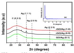
Fig. 2: XRD patterns of GO (a) and Ag-rGO nanohybrids prepared with different concentration of GO (0.1, 0.5, and 1.0). Inset: XRD pattern of GO sheet.
