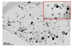
Fig. 4: TEM image of GO–Ag nanohybrid. Inset: Image at higher magnification.
