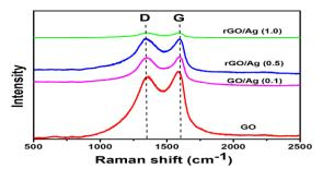
Fig. 3: Raman spectra of GO and Ag-rGO nanohybrid with different concentration of GO.
