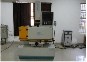
Figure 1: Electric Discharge Machine
