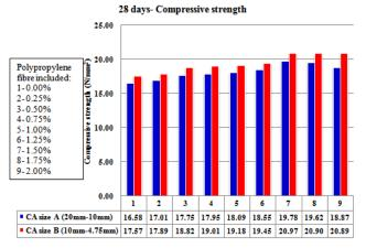
Fig. 1:Compressive Strength Of Fibre Included Pervious Concrete.
