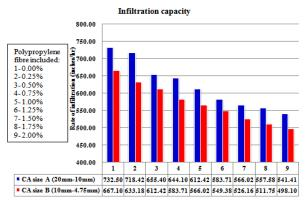
Fig. 4:Infiltration Capacity of Fibre Included Pervious Concrete.
