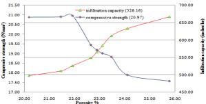
Fig. 5: Relationship between Compressive Strength, Porosity and Infiltration Capacity.
