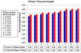
Fig. 3:Flexural Strength of Fibre Included Pervious Concrete.
