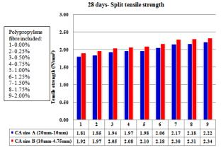
Fig. 2:Tensile Strength of Fibre Included Pervious Concrete.
