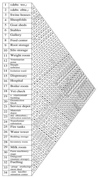
Fig. 4: Principles of cooperation and blocking of buildings and structures matrix:
