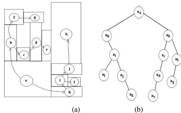
Figure 1: A packing represented by B\*-tree
