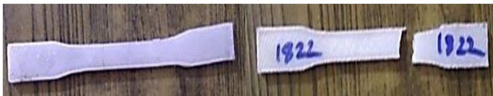
**Fig. 11:** Tensile Specimen after Testing (PET-G).
