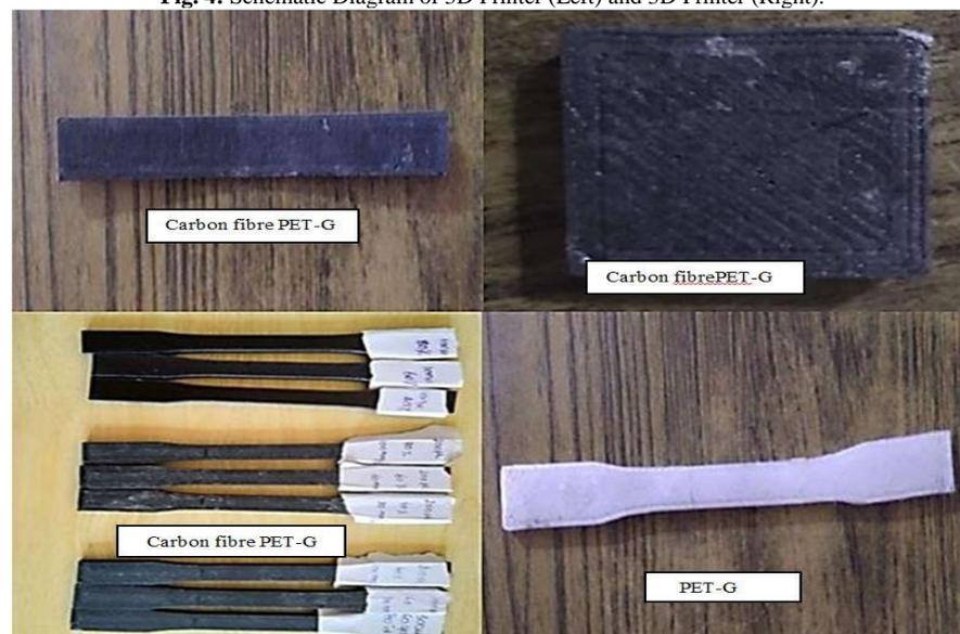
Fig. 5: 3D Printed Specimen before Testing.
