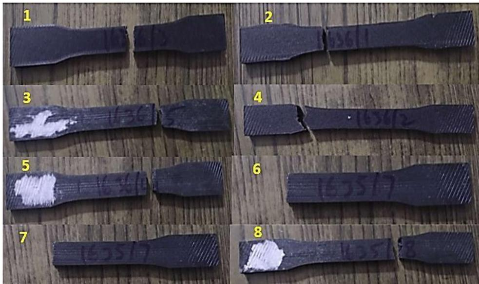
**Fig. 10:** Tensile Specimens after Testing (Carbon Fiber PET -G).
