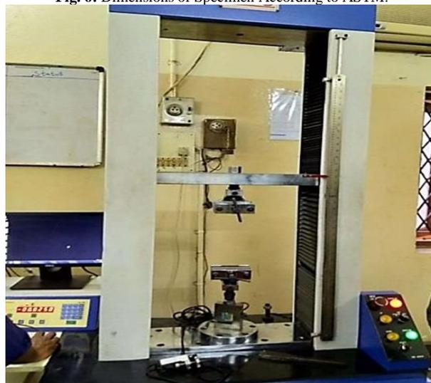
**Fig. 7:** Mechanical Tests Conducted on 60T UTM (Tensile Test).
