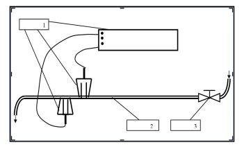
**Fig. 1.** Stand for the preparation of magnetized water: 1 - device "Ilios-M"; 2 - plumbing; 3 - valve
