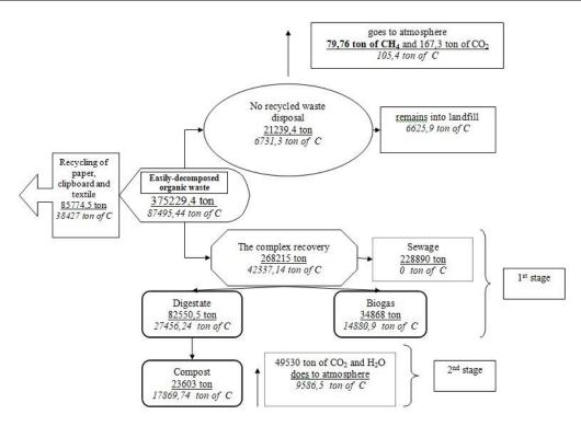
Fig. 3: The mass balance during the complex recovery of organic waste part of MSW
