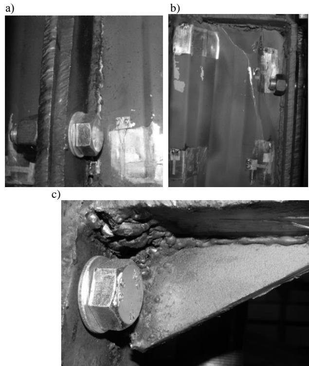
Fig.7: Forms of bearing capacity loss in experimental tests of series 2 samples: a), b) the rupture of the weld in the areas near the flanges; c) the separation plate (fixing flange beams to the shelf)
