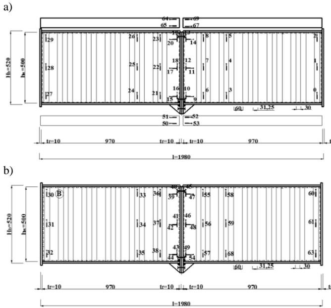
Fig.4: The layout of strain gauges in experimental samples B3 and B4
