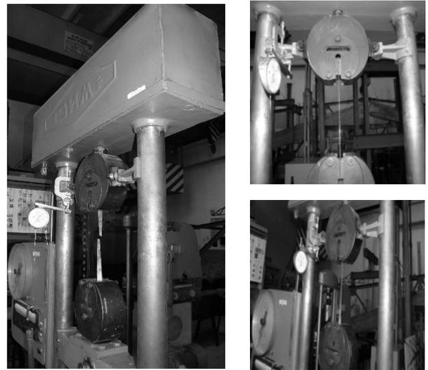
Fig.5: Tensile testing of flat samples
