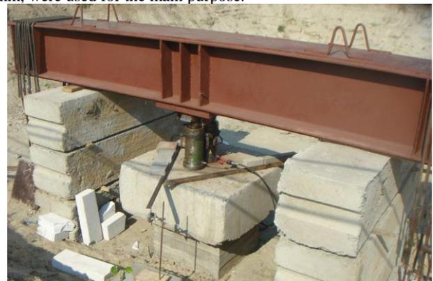
**Fig. 6:** Static pressure bench testing by means of jacks, cargo beam and two anchor piles.
