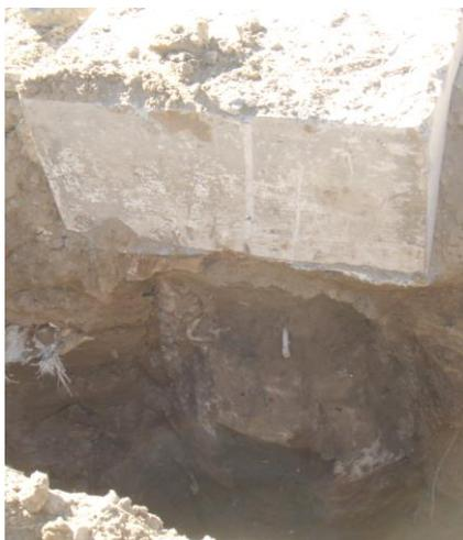
**Fig. 9.** Investigation of the destruction vibroreinforced soil-cement pile №3
