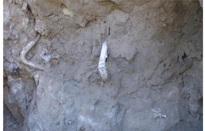
**Fig. 10:** Loss of local resistance of three reinforcing bars of a frame during static testing of vibrated reinforced cement pile №3
