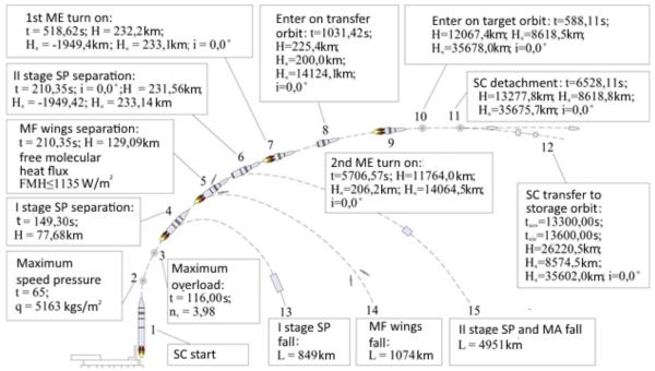
Fig. 1: Stages of spacecraft launch into orbit scheme: SP – structure part, which is separated; MF – main flyer; MA – middle adapter; ME – march engine; H – flight height;  $H\pi$  – perigee height;  $H\alpha$  – apogee height; i – tilt; t – flight time; tst – spacecraft transferring to storage orbit start time; tend – spacecraft transferring to storage orbit end time; L – approximate fall distance from the launch point.
