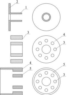
**Fig. 5:** Discharge device design: 1 - electrode holder isolation; 2 - face isolation; 3 - rod electrodes guide; 4 - metal electrode holder; 5 - electrode insulator
