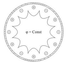
Fig. 6: Localized discharge gap electrostatic field geometry: "+" - rod anodes; "-" - rod cathodes
